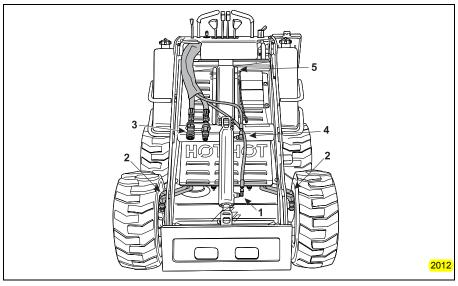
Figure 4–7 Inspect Hydraulic Lines and Fittings
